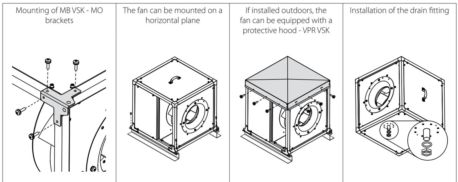
The MK VSK brackets and the VPR VSK protective hood are not included in the delivery set and must be ordered separately.
