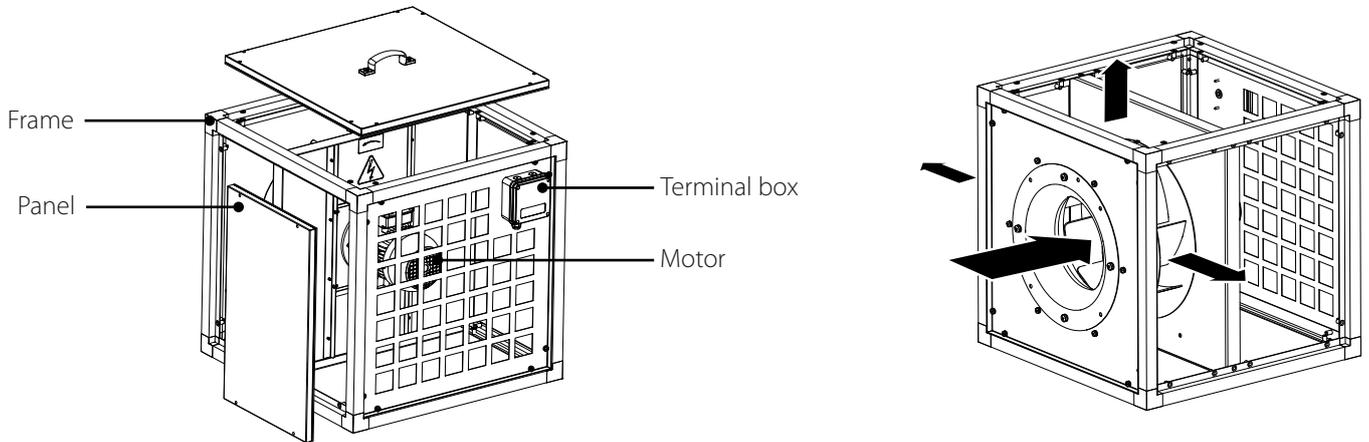
When connecting the fan to the air duct system, it is recommended to use the accessories specified in the User's manual.
