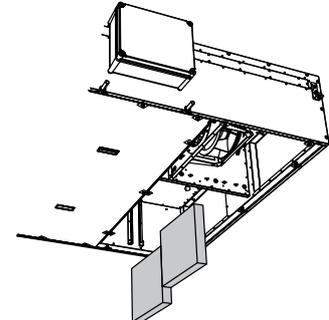
Remove the service panel to access the heat exchanger. Pull the heat exchanger out. Disconnect the connector from the bypass damper actuator. Disconnect the bypass unit and pull the second heat exchanger out.
