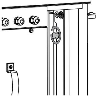
Remove the two butterfly bolts that fix the retaining clamp.
