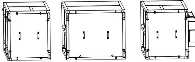
Prior to mounting the unit, connect the sections and fix them with screw connections.
