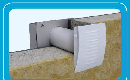
Mounting into a thin wall using the EH-2 outer hood
